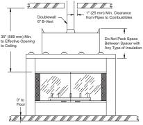
Figure 4 - Clearances from Side View
